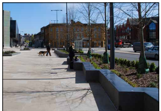
Figure 35: Narrower lane widths has allowed the creation of wide spaces for shared cycle/pedestrian footpaths, seating and planting. Raised planting areas help to define pedestrian and cycle paths and offers opportunities for informal seating. (Frideswide Square, Oxford).
