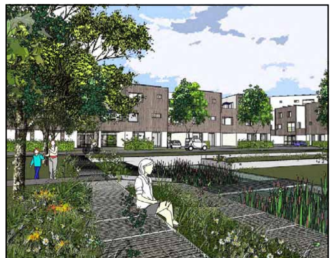
Figure 51: Reed bed ponds help to slow the flow and clean water. Quad, Great Kneighton, Cambridge.
