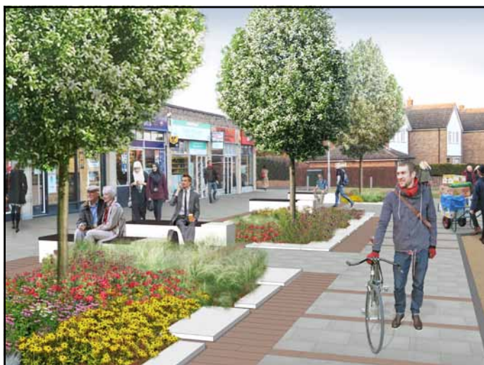
Figure 50 - Rain garden planted with trees and planting which can withstand drought and occasional flooding. Currently under construction at Rectory Terrace, Cherry Hinton High Street, Cambridge.
